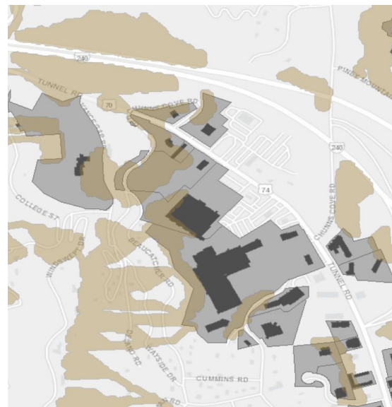
NCDEQ debris flow pathways with properties exposed to landslides.
